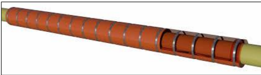
Figuur 2.5.2: URADUCT® beschermingslaag rondom kabel ( https://www.trelleborg.com/en/offshore/products--and--applications/subsea--operations--protected--by--njord/njord--protection/uraduct--range/uraduct )
