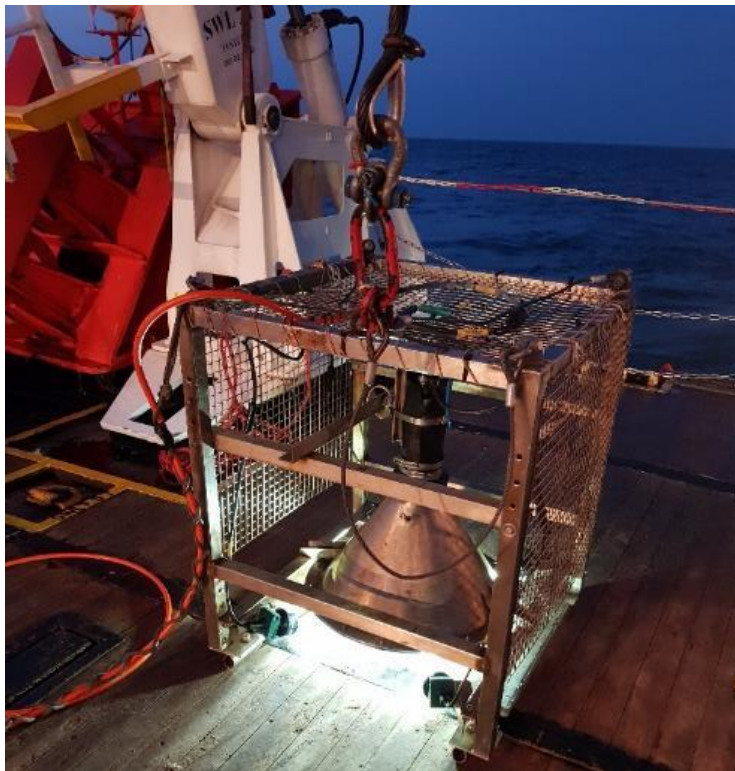
Figure 3.7 Drop Down Video system rigged for deployment.
