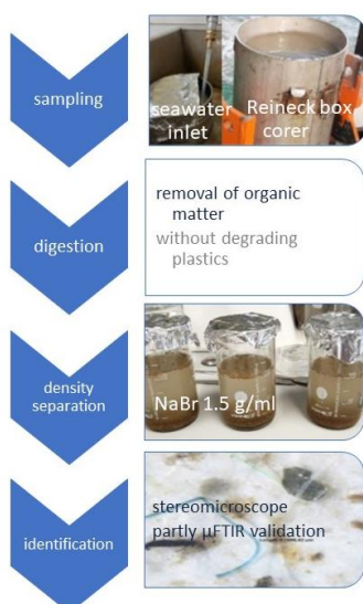
Figure 3 Generalized overview of methodological protocol for microplastic analysis
