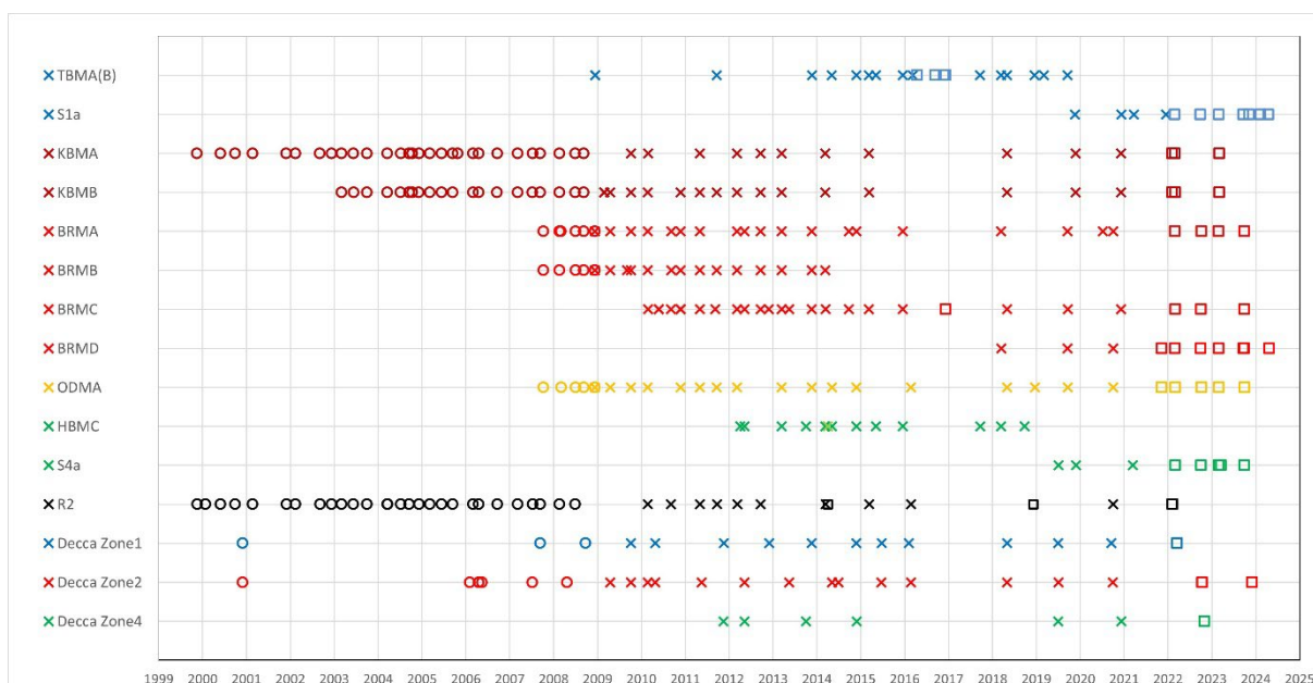
Figure 3. Completed timeline of the different MBES surveys of the monitoring zones and Decca reference lines. Bathymetric and BS data acquired with MBES EM1002 (round) and EM3002 dual (cross) onboard RV Belgica, and EM2040 dual RX (square) onboard RV Belgica, RV Simon Stevin and Geosurveyor XI.
